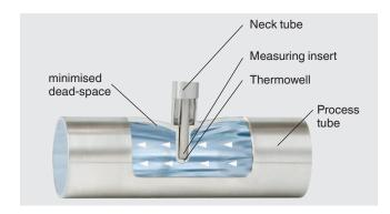
The patented (patent No. DE 102010037994 and US 12 897.080) hygienic design of the TW61 flow-through housing enables dead-space minimised, invasive temperature measurement and a flexible mounting position through self-draining.
