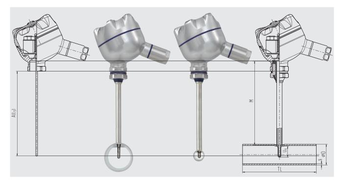
Due to the variable neck tube length M, measuring inserts with standardised insertion lengths A (I<sub>1</sub>) can be used. Thus, variance and stocking of spare parts are minimised. At the same time, the use of correct insertion lengths in the event of replacement is ensured.
