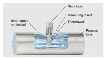
The patented (Patent No. DE 102010037994 and US 12 897.080) hygienic design of the TW61 flow-through housing enables dead-space minimised, invasive temperature measurement and, through self-draining, a flexible mounting position.
