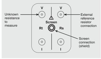
The BNC input connectors are located to the left of the display. The central connector is used when a screen connection is required. The two right-hand connections are only used when an external reference resistor is selected;
