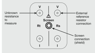
The BNC input connectors are located to the left of the display. The central connector is used when a screen connection is required. The two right-hand connections are only used when an external reference resistor is selected;
