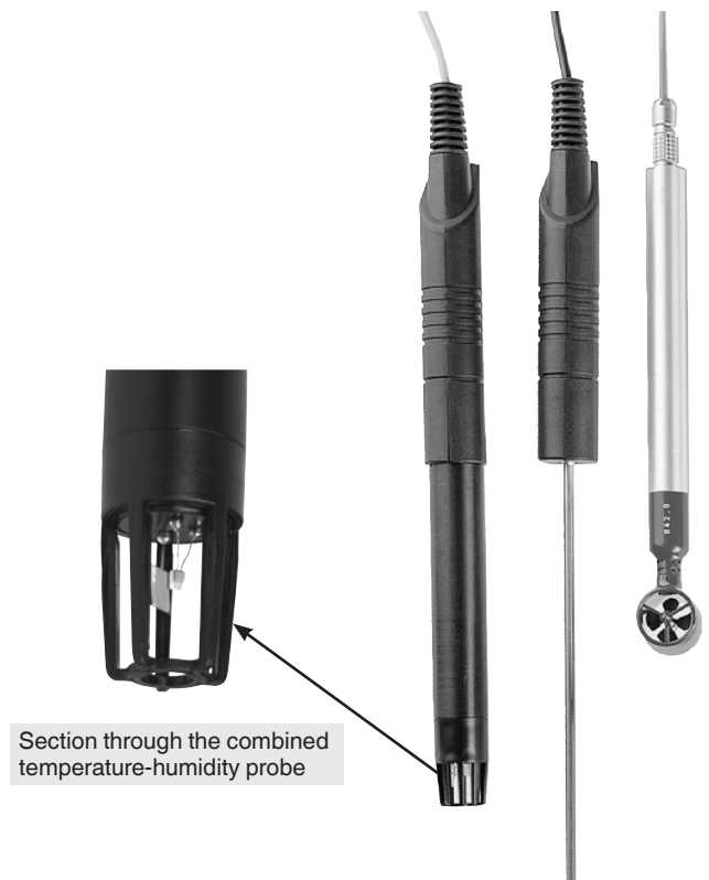
Fig. left: combined temperature-humidity probe Fig. centre: immersion probe Fig. right: vane flow sensor
