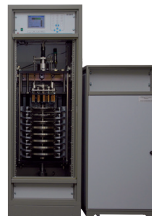
Automatic pressure balance, model CPB8000
