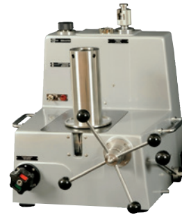
Primary-standard pressure balance, series CPB6000
